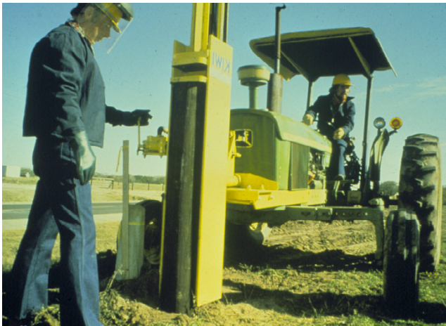
Figure 11. A tractor-mounted post driver.
