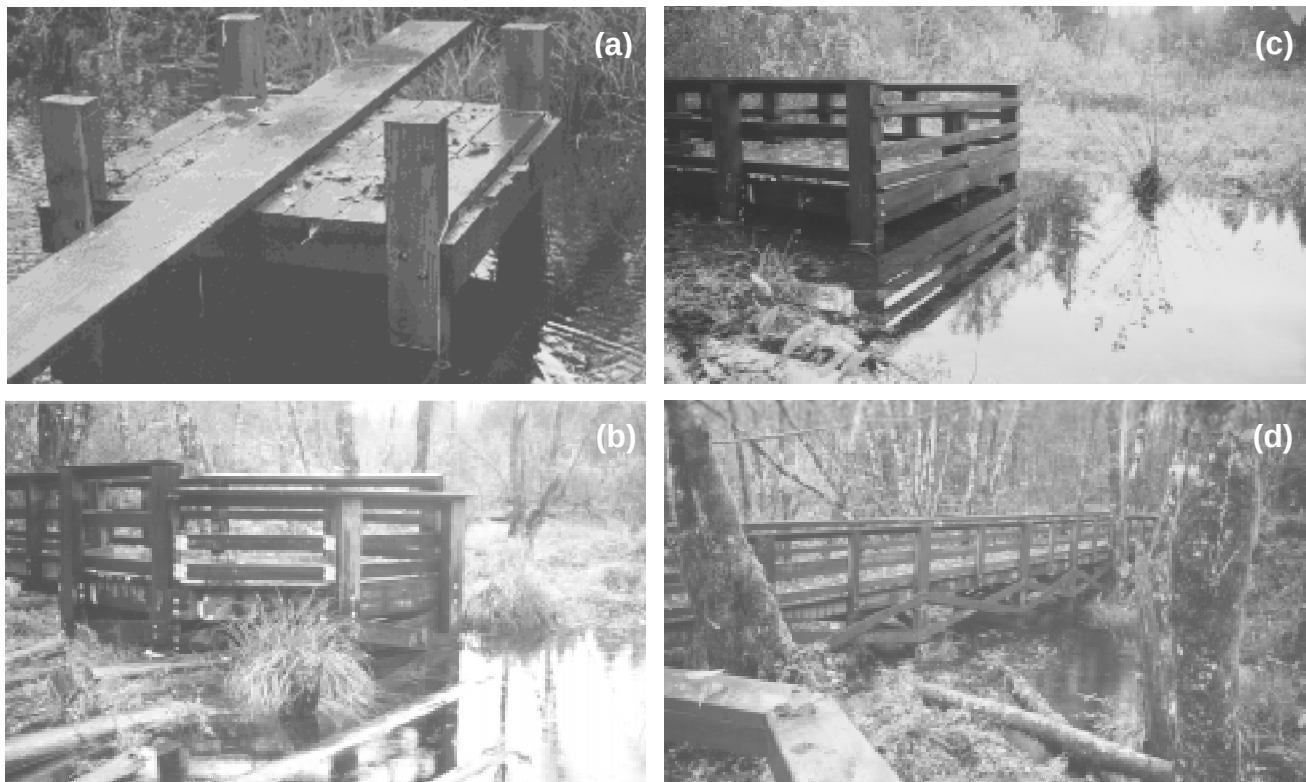
Figure II-3—Control and treatment sites for Wildwood wetland study, 1996–1977. (a) Mechanical control site; (b) ACZA-treated wood viewing platform; (c) ACQ-B-treated wood viewing platform; (d) CCA-C-treated wood bridge.
